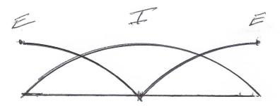
The two curved lines shown are the (E) for the voltage field and the (I) for the current field. From Ohm's law, we know that in a DC circuit, R=E/I. In an AC or RF circuit, the "R" is replaced with the symbol "Z", for Impedance. Thus, Z=E/I.
